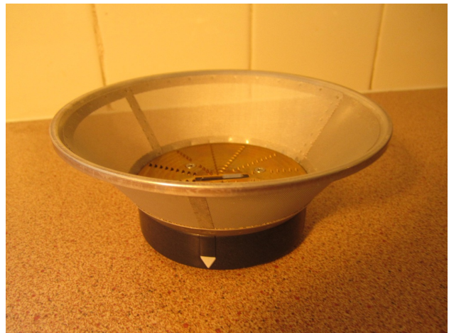
The engine causes the strainer to spin at a very high speed. The centrifugal force causes the juice to pass through the strainer and make its way into the jug.
